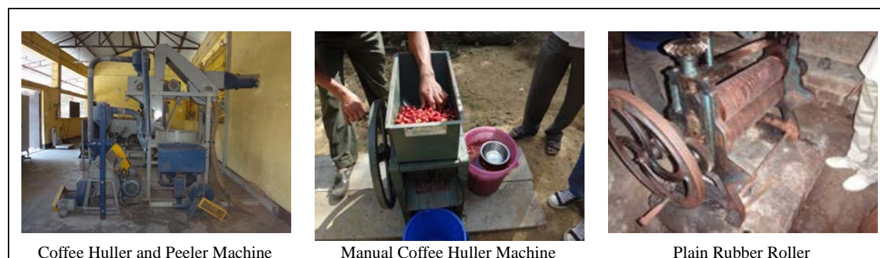
Photo 4.5.2 Post-harvest Processing Machines for Coffee and Rubber
