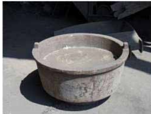
Aluminum extracted by ash squeezing
