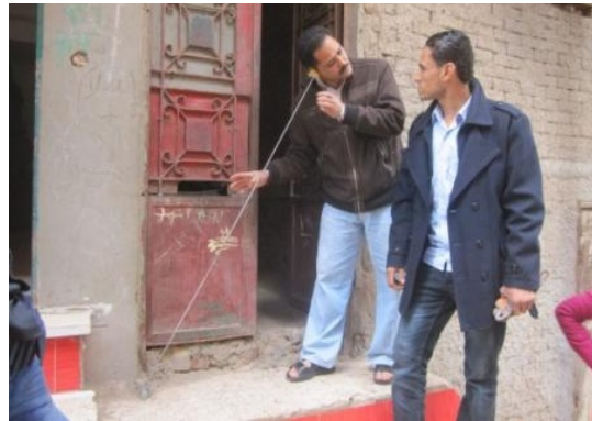
Figure 4.2-3 House Connection Survey using Acoustic Rod on GHAPWASCO
