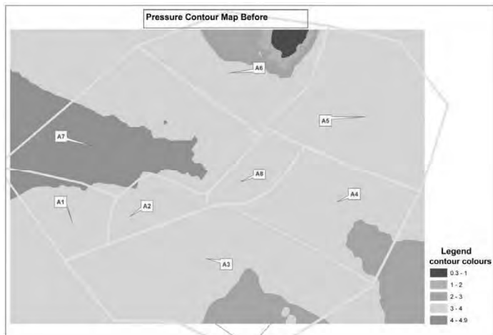
Figure-4 Pressure Contour Map before Isolation
