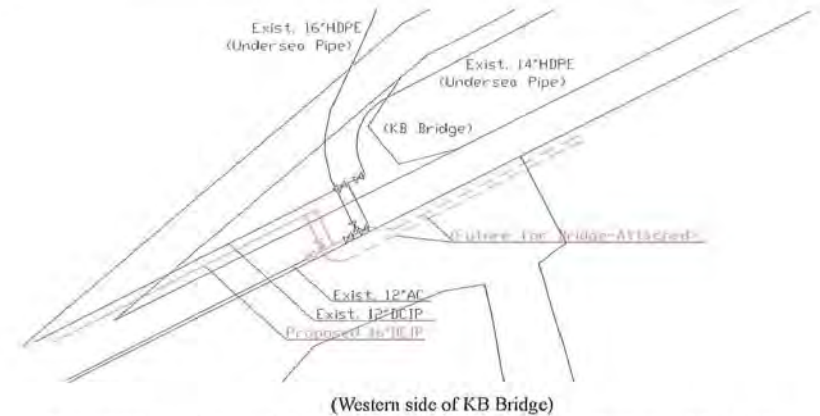
Figure 2.2.1-3 Proposed Connections to Existing Undersea Pipeline around KB Bridge
