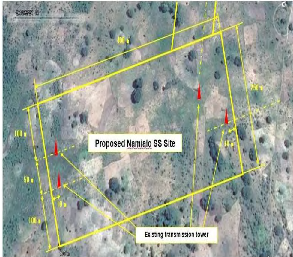
Figure 1- Map of Namialo Substation proposed Site
