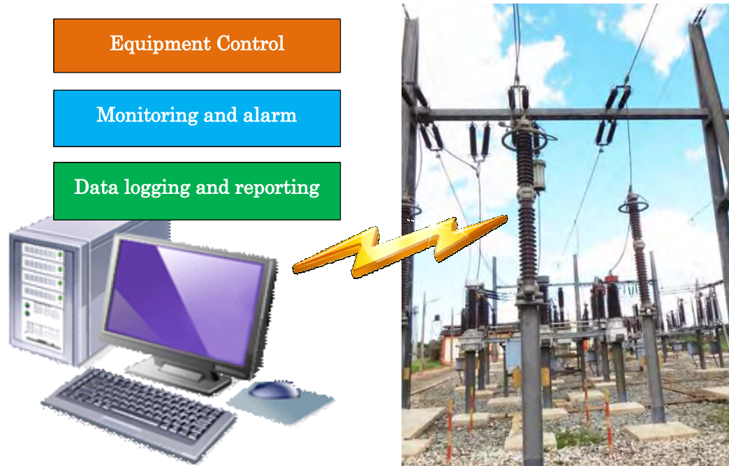
Figure 2-11 Conceptual diagram of SCADA system
