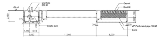
SEPTIC TANK & SEEPAGE PIT SECTION
