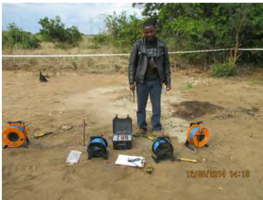
Figure 4 - SEV set-up and geophysical technician during the field works near Borehole 01
