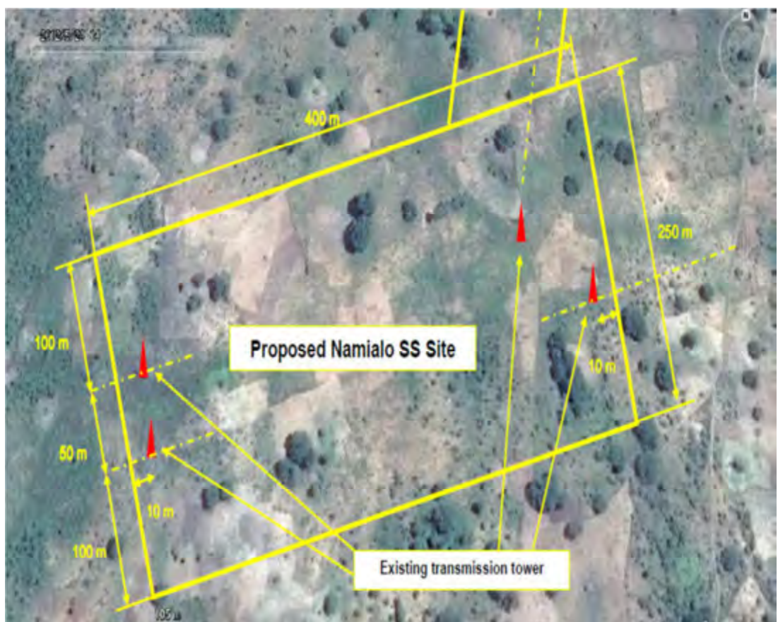
Figure 2: Layout of Namialo Substation Site
