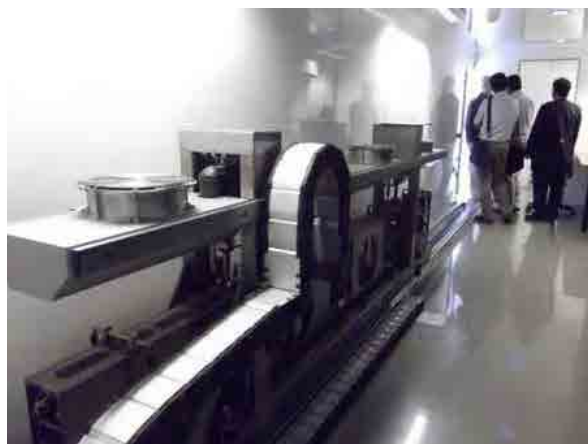
Traffic Speed Deflectometer (内部)
