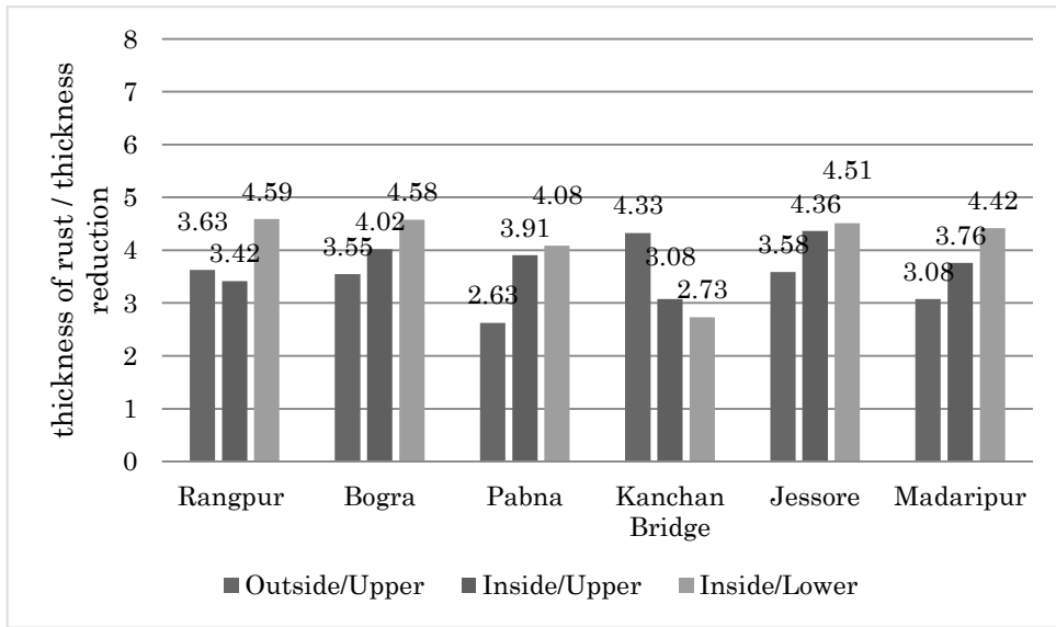
Figure 1 The Ratio between Thickness of Rust and Corrosion Loss after Half Year
