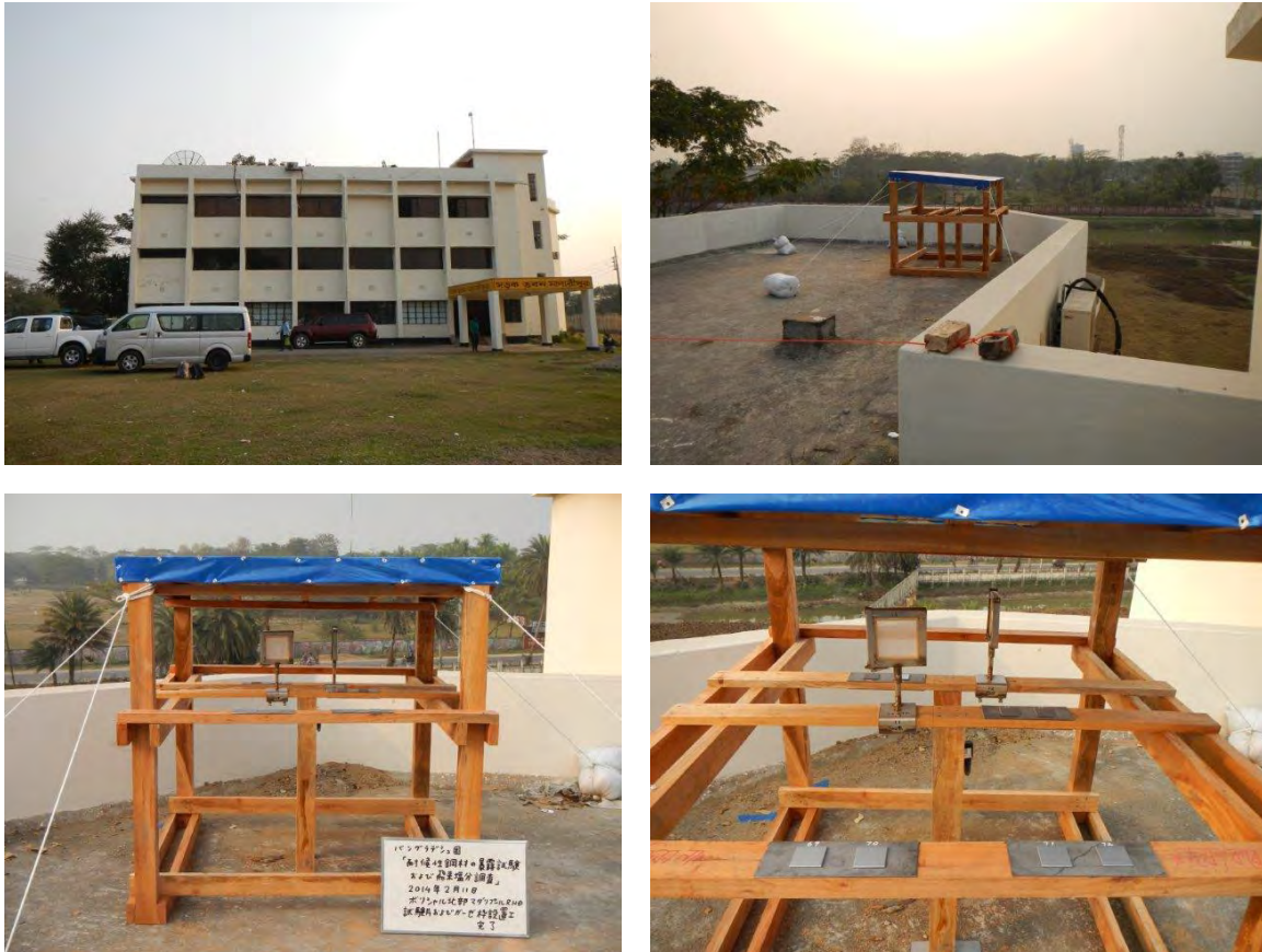
Figure 8.4.3 Installation of Test Specimens on Office Rooftops
