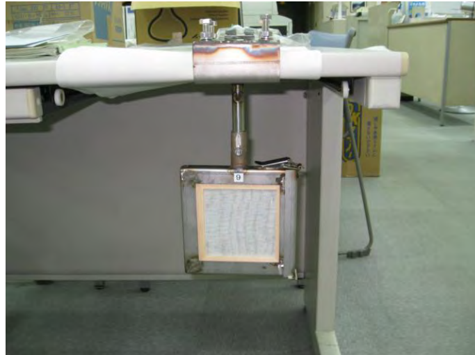
Figure 8.4.1 Gauze Frame for Airborne Salt Test
