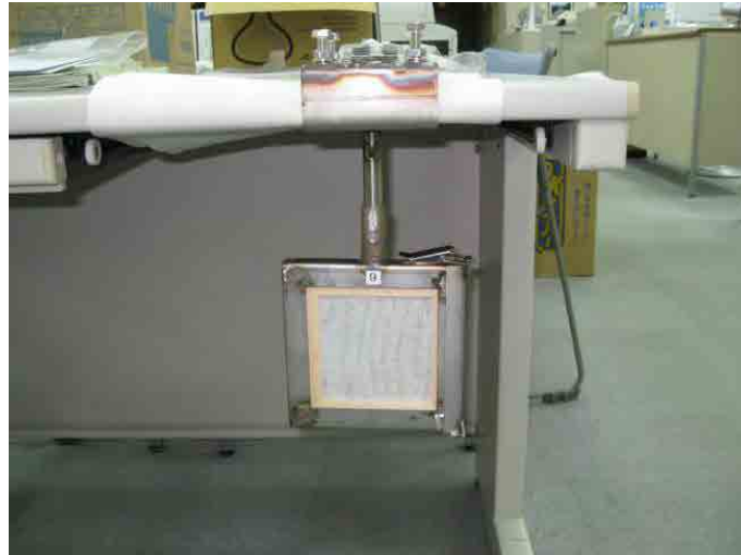
Figure 8.4.1 Gauze Frame for Airborne Salt Test
