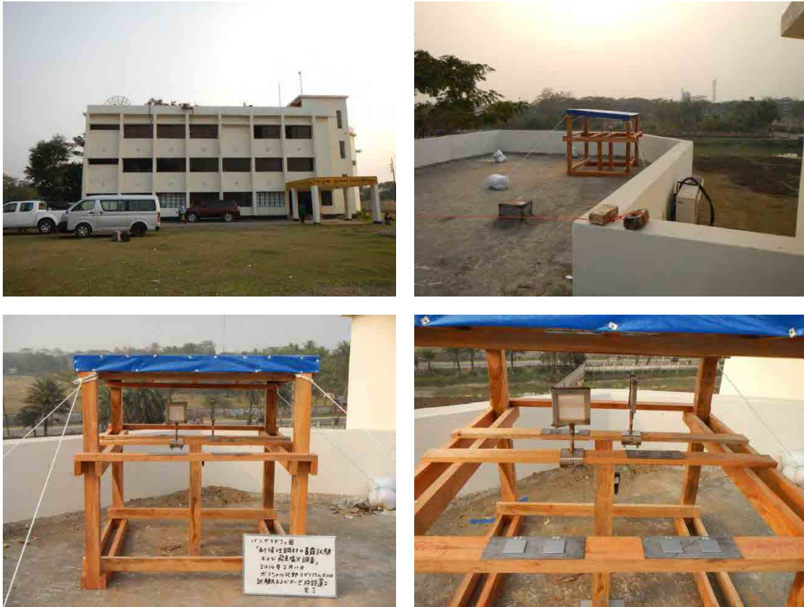
Figure 8.4.3 Installation of Test Specimens on Office Rooftops
