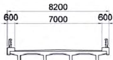
The curb width and the handrail are applied to Japanese Standard.
