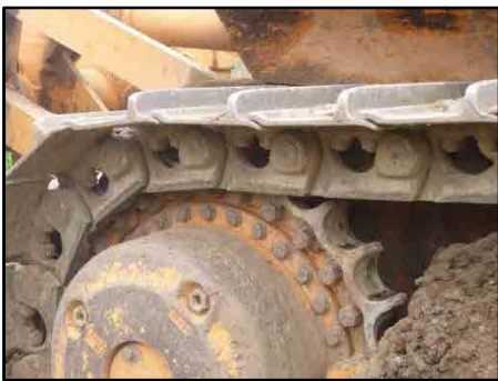
Wear condition of undercarriage (Bulldozer)
