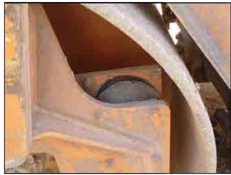
Vibration absorbing rubber of 10ton vibration roller
