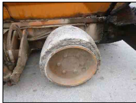
Wear condition of front tire (Asphalt finisher)
