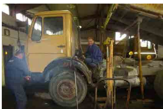
Photo 3-4 Transmission installation work (Bitola)
