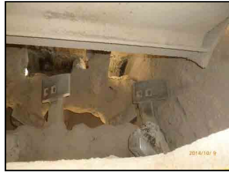
Almost no wear in the mixer chip
