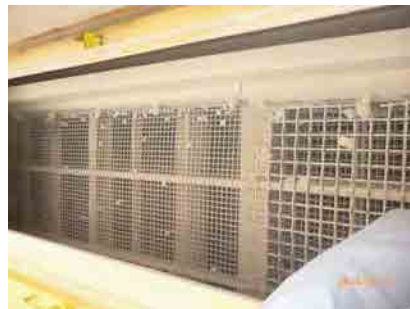
Screen of Vibrating sieve (still workable)
