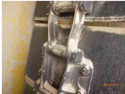
Bucket chain of hot elevator (quite few wear)
