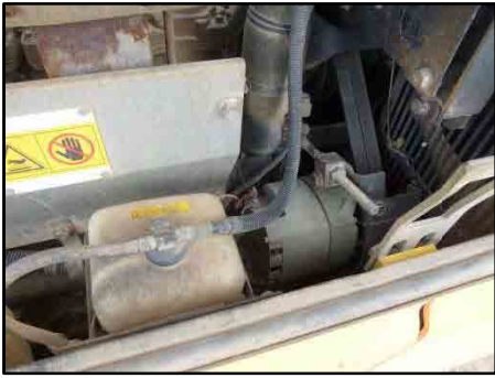
Locally purchased alternator (Bulldozer)
