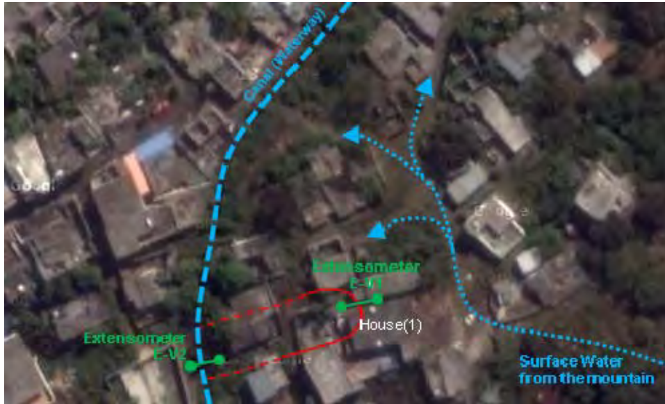
Photo 3.7.92 Landslide Plan Map, 2nd Reconnaissance at, 22nd February 2013 (source: JET)
