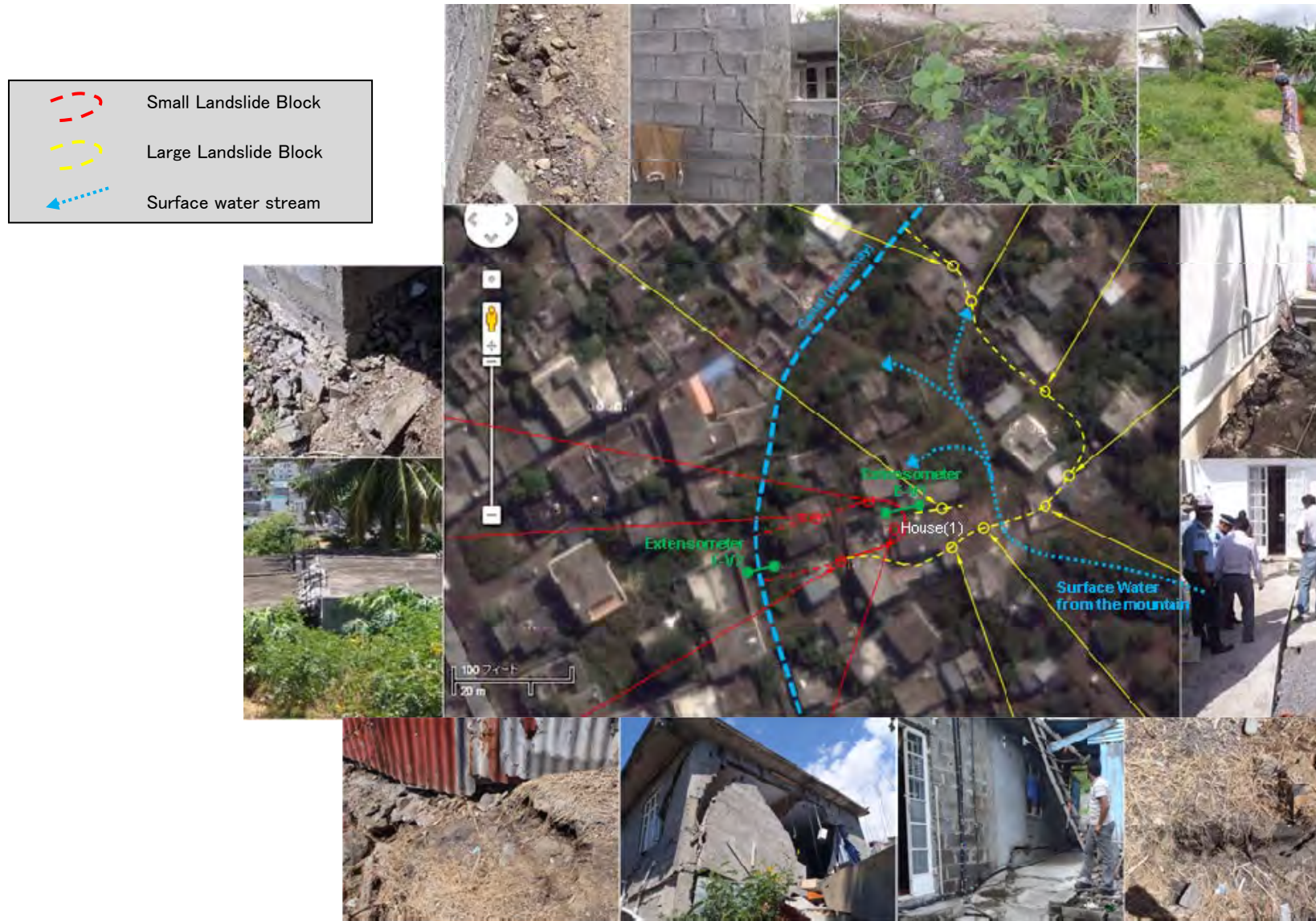
Figure 3.7.7 Landslide Plan Map (3rd Reconnaissance on 26th February 2013) (source: JET)
