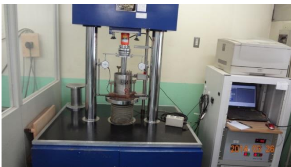
Measuring by CBR Test Device
