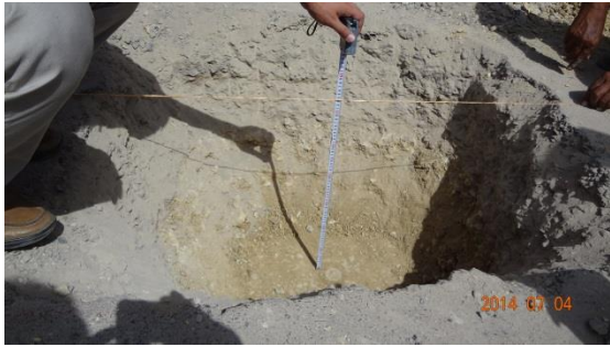
Excavation Cross Section(Depth 63cm, Subgrade thickness 33cm)
