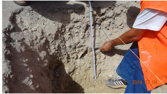
Excavation Cross Section(Depth 63cm, subgrade thickness 33cm)
