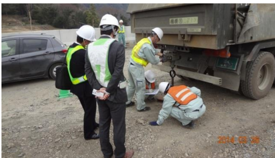
In-Situ CBR Measurement
