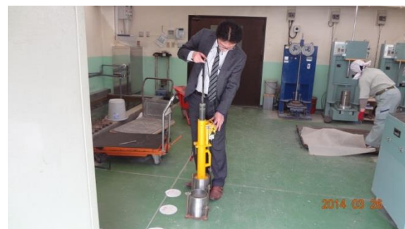
Test of Material Compacted by CIST
