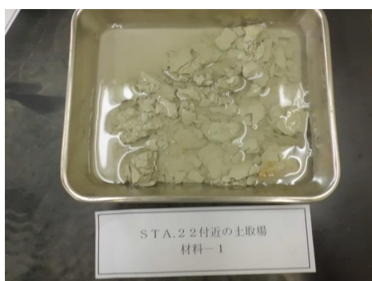
Grain micronizing of material-① after 18 hours of absorbing of water and swelling
