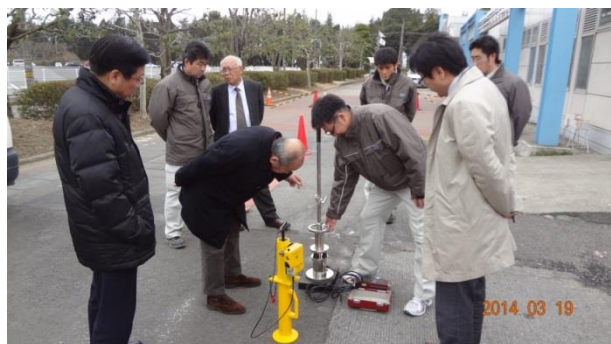
Measurement by an Easy FWD Device
