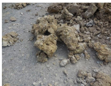
Cement Stabilized Sub-base of Clay
