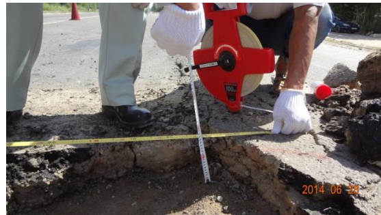
⑥ Pavement Thickness 10mm
