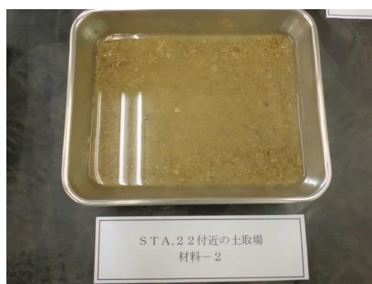
Grain micronizing of material-② after 18 hours of absorbing of water and swelling
