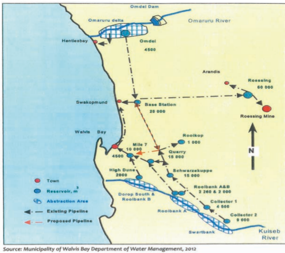
Figure 5.18: Water scheme in coastal area
