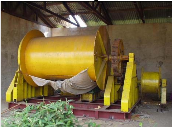
Photo C.2.19 No.7 Hauling Winch
