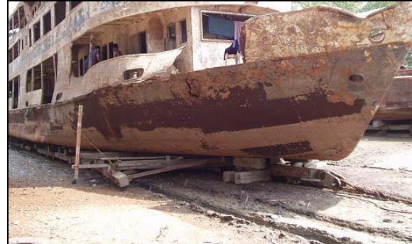
Photo C.2.2 Damaged Wooden Cradle
