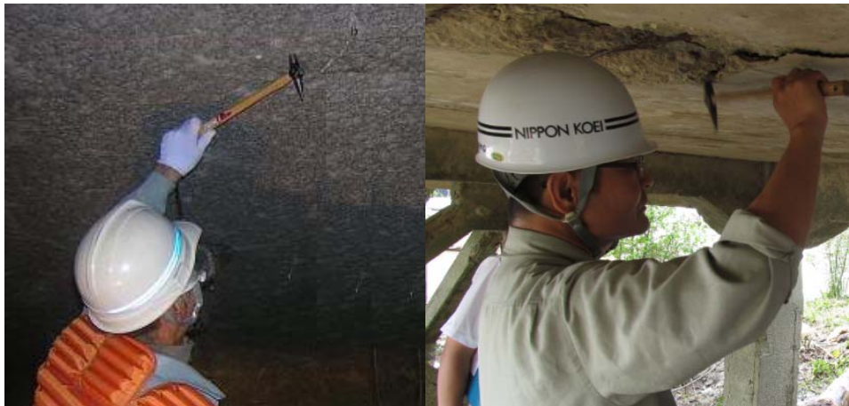
Photo 13.4.6 Hammering Test (Spalling and Delamination)
