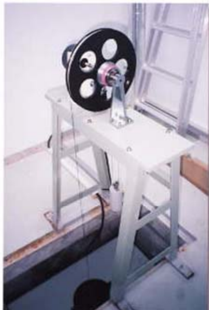
Photo 12.5.1 Tide Gauge with Float System
