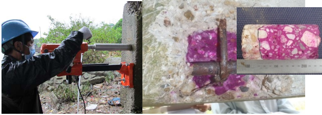
Photo 13.4.9 Core Sample and Chipping Concrete
