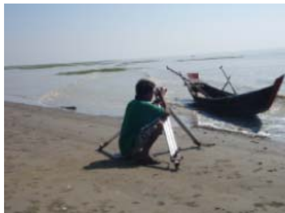
Figure 11.8.22 Recording of Water Level by Transit at Intervals of Ten Minutes
