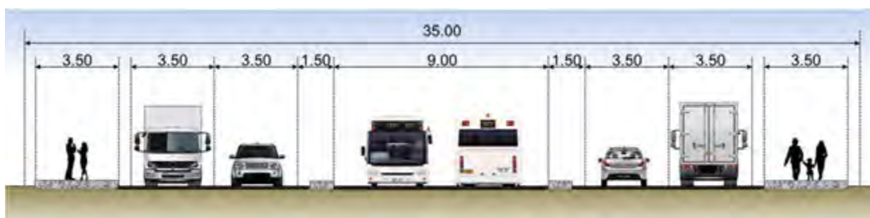
Figure 3.5 Proposed Typical Cross Section for Secondary Roads
