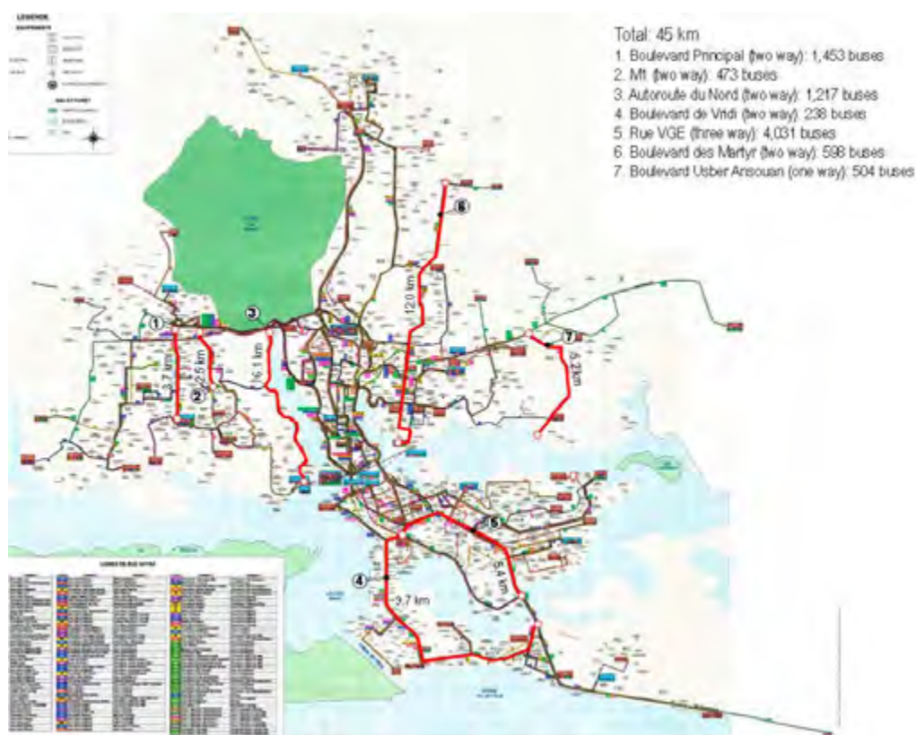
Figure 4.9 Development of Dedicated Bus Lanes in Abidjan
