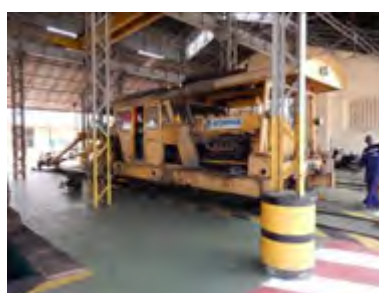
Ballast tamping machine.
