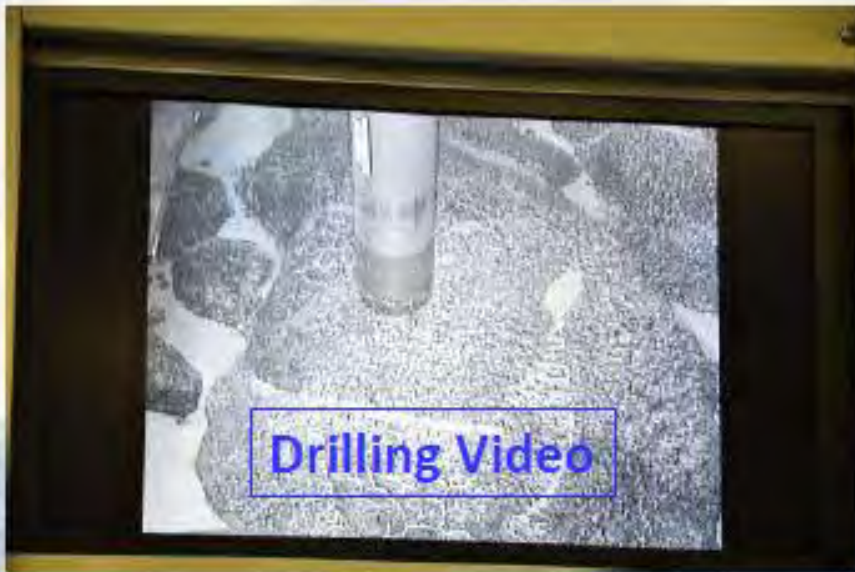
Drilling operation observed by high vision TV camera mounted on the BMS
