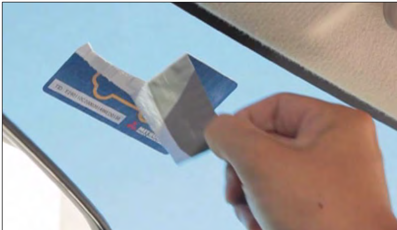
Figure 8-3-3 Tamper Proof function of RFID-Tag (Image)
