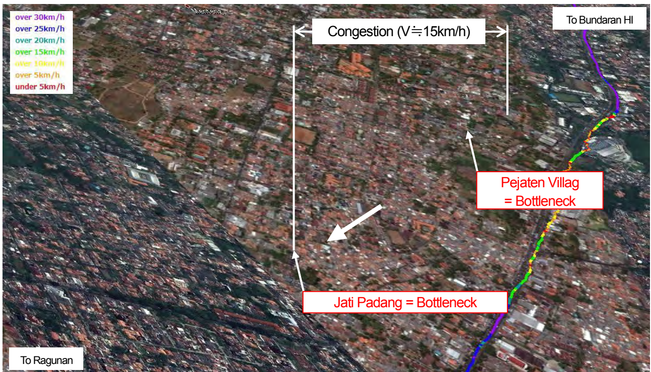
Figure6-3-5 Major Bottlenecks (Corridor 6 / Westward : Bundaran HI→Ragunan)
