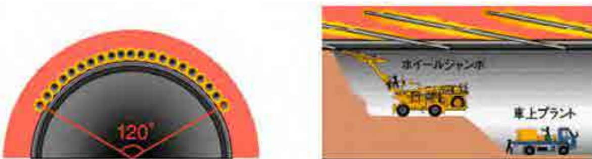
FIGURE 9.6-2 IMAGE OF EXECUTION OF LONG SPAN FORE-PILING
