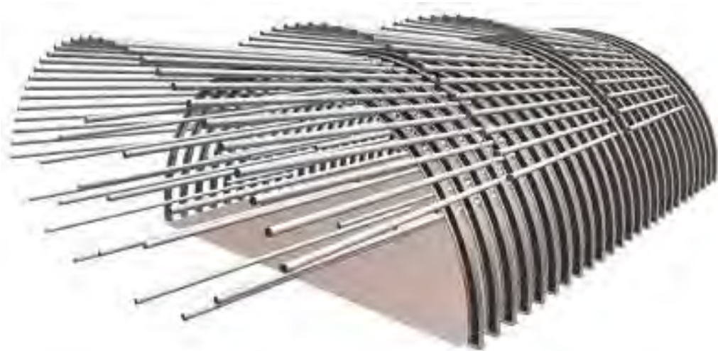
FIGURE 9.6-1 LONG SPAN FORE-PILING IN DIFFICULT GROUND
