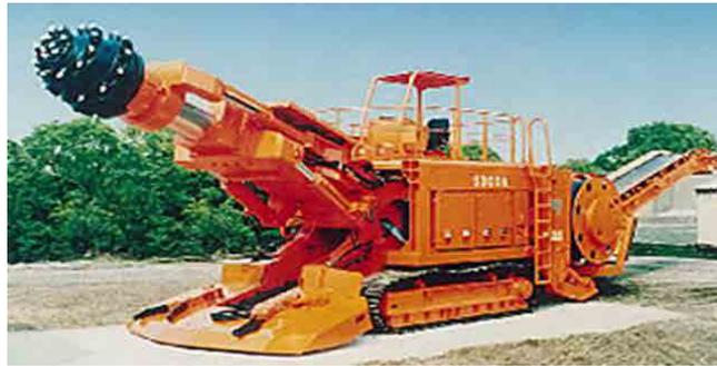
**Excavation Machine: Road Header**
