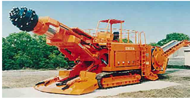
Excavation Machine: Road Header
