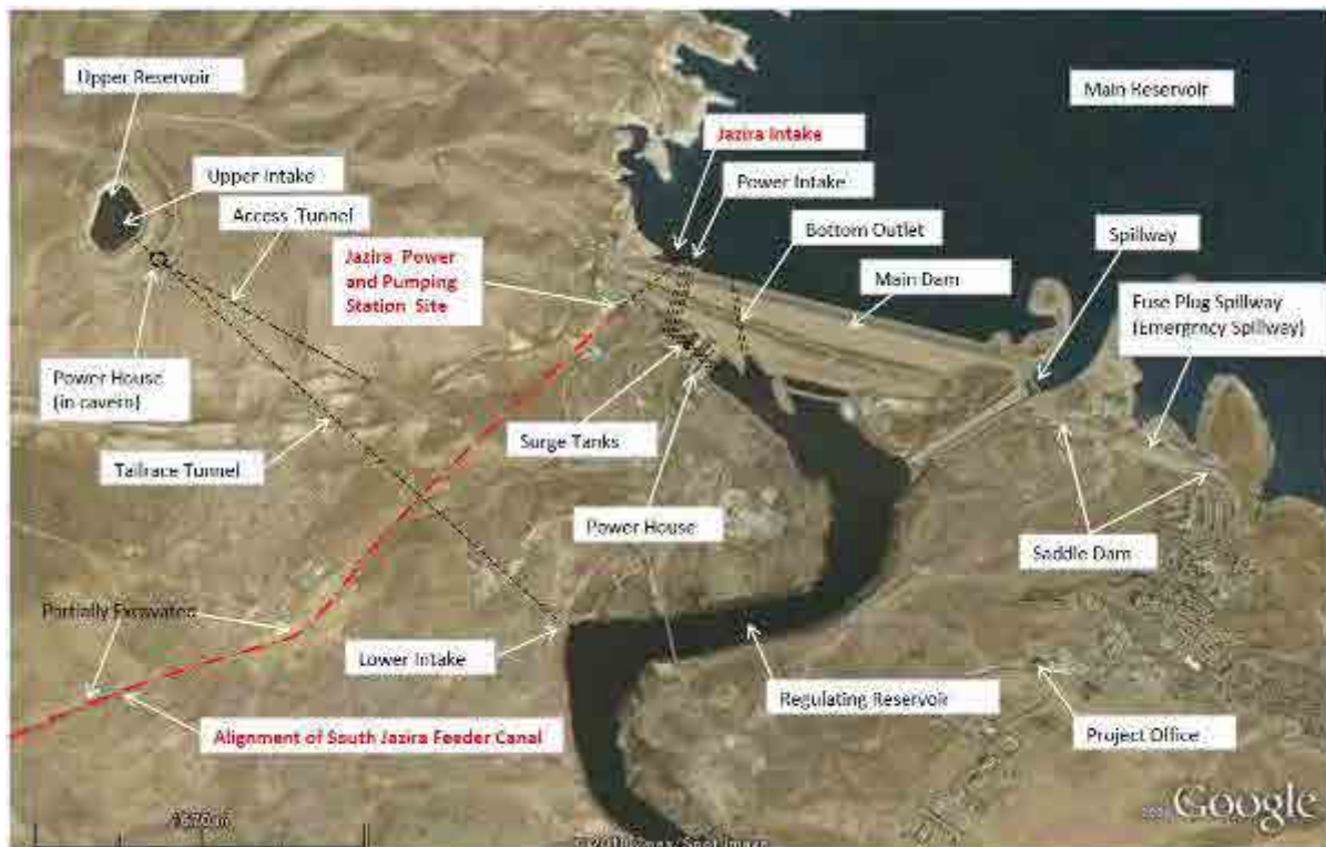
Fig. 3.6-1 Layout of Main Structures of Mosul Dam
