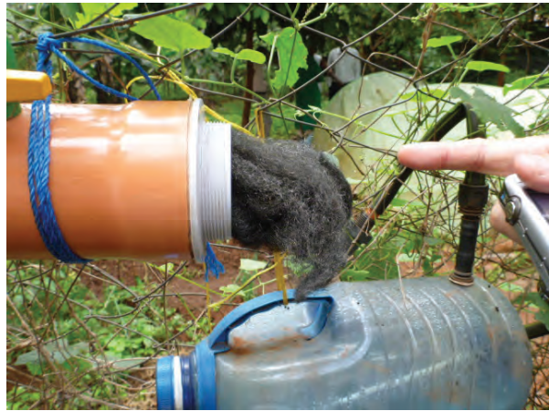
Steel Wool for H 2 S Removal
