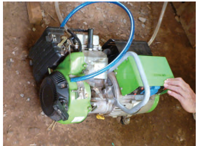
Petro Engine Generator
