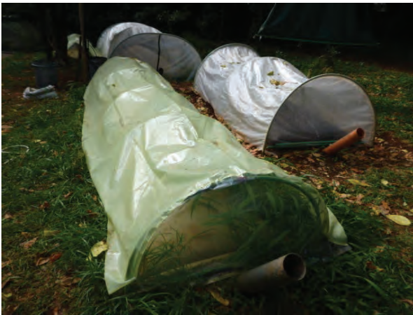
Digester with Greenhouse Cover
