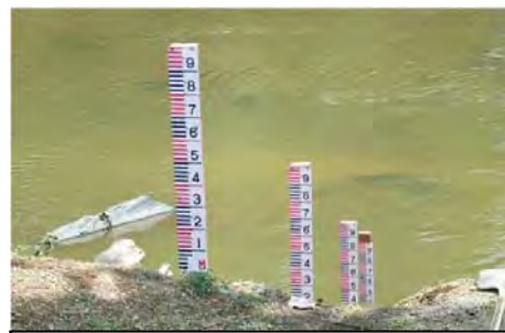
Stepped water level gauge
