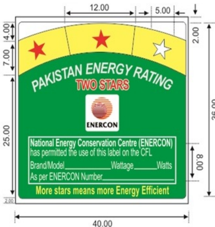
Figure-3: Dimensions of the Energy Efficiency Rating Label (all values in mm)
