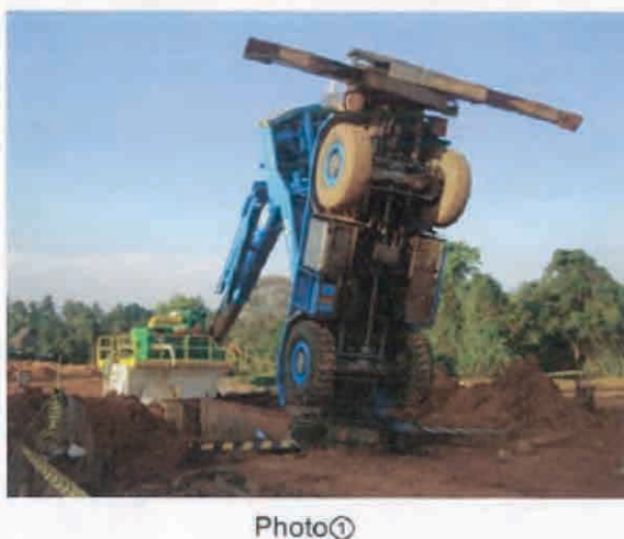
Fig. 4.4.18 Accident Caused by a Topped Crane
