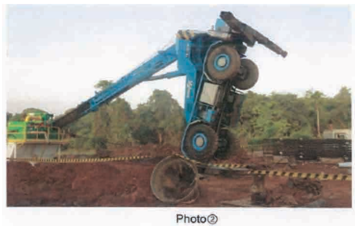
Fig. 4.4.18 Accident Caused by a Topped Crane
