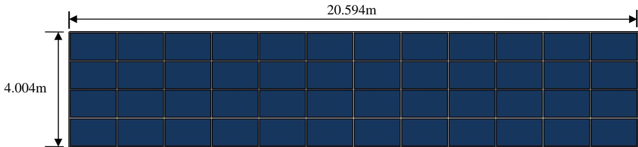
Figure 3.3.7-9 PV array size (projection of horizontal surface)
