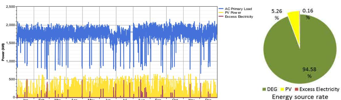
Figure 3.3.6-12 PV deployment simulation (1200-800kW)
