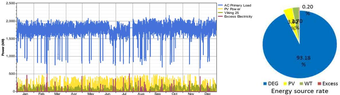
Figure 3.3.6-14 DEG-PV-WT hybrid system simulation
