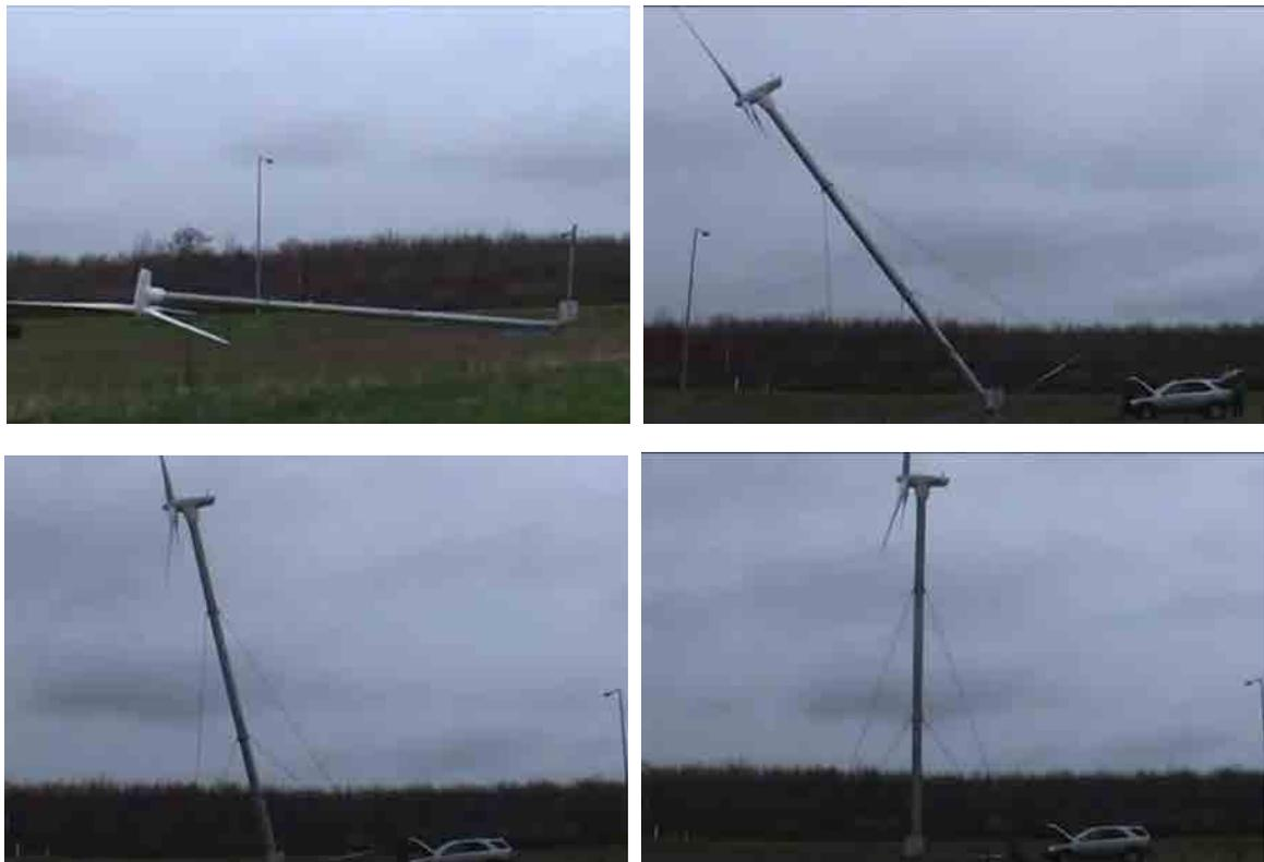
Figure 3.3.3-11 Wind turbine retraction conditions
