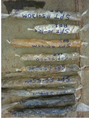
Figure 3-4: SPT cores from BH1
