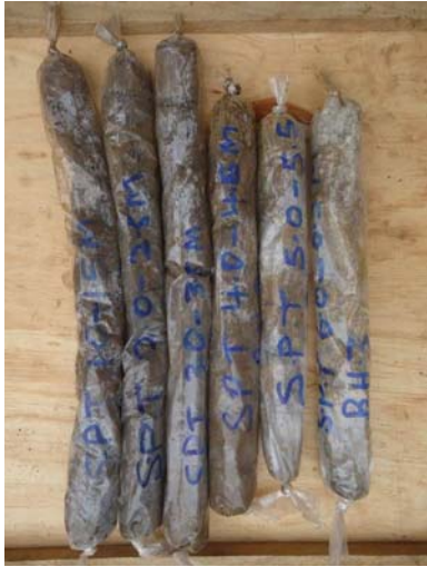
Figure 3-10: SPT cores from BH3
