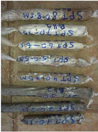
Figure 3-7: SPT cores from BH2
