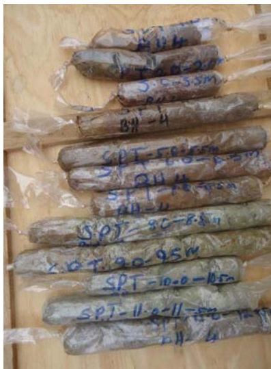
Figure 3-14: SPT cores from BH4
