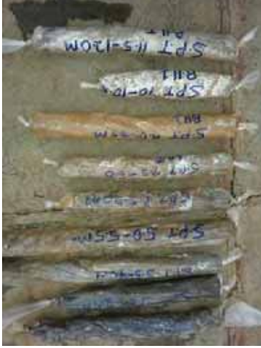
Figure 3-4: SPT cores from BH1
