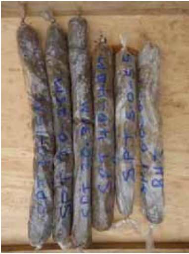
Figure 3-10: SPT cores from BH3
