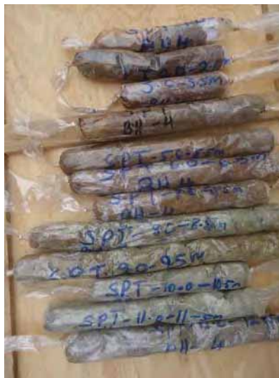
Figure 3-14: SPT cores from BH4
