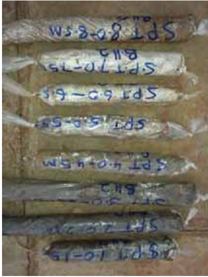
Figure 3-7: SPT cores from BH2
