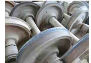
Worn tires are reused by overlay welding
