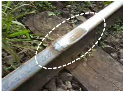
Wheel burn ( Kojokrom ~ Angu section)
