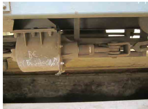
Photo 4.2.124 Check of Function under Active Brake Cylinder
