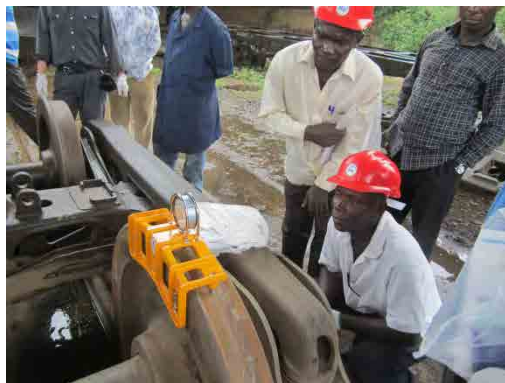
Photo 4.2.107 Measurement of Wheel Diameter
