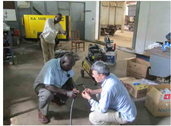
Photo 4.2.86 Brake Test Equipment Components (Assembling air hose joints purchased in Ghana)
