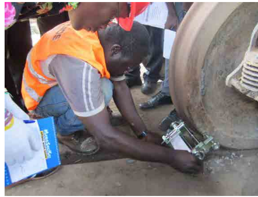
Photo 4.2.112 Measurement of Wheel Tread (Practical training)
