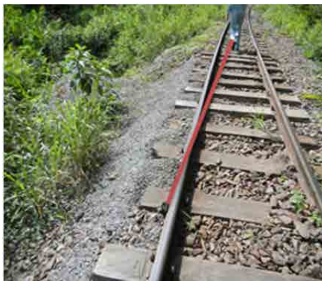
Photo 2.3.9 Trace of Derailment (1)
