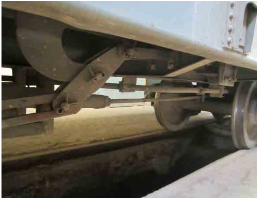
Photo 4.2.133 Unlubricated Brake Lever
