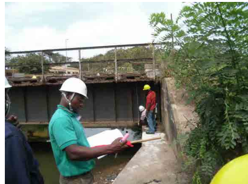
Photo 4.2.23 Measurement of Beam Height
