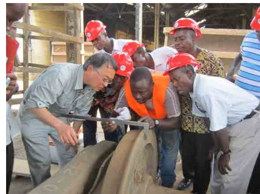
Photo 4.2.108 Measurement of Wheel Thickness
