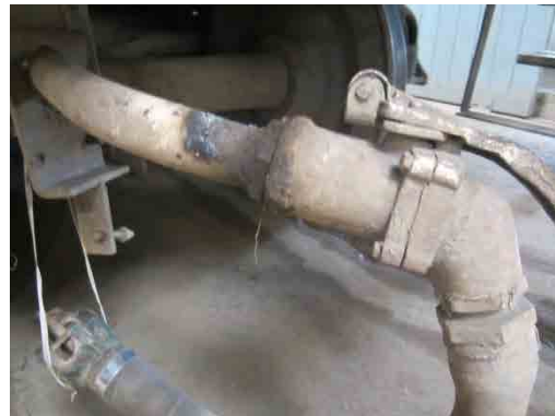
Photo 4.2.94 Repair of Brake Pipe from Air Leakage
