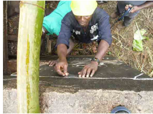
Photo 4.2.15 Measurement by Crack Gauge (2)
