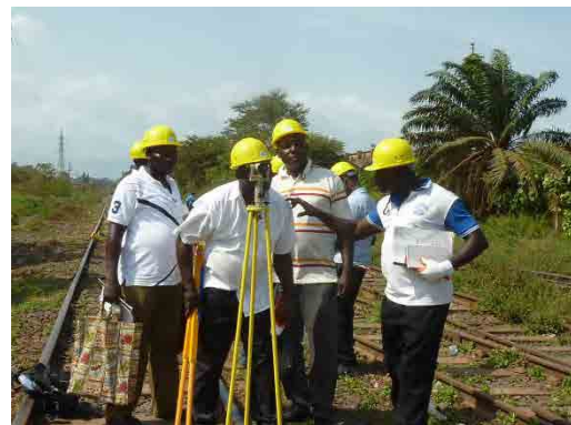
Photo 4.2.59 Trainees are measuring the longitudinal level of the rail surface by using the level measuring equipment
