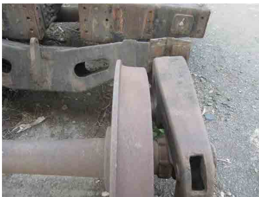
Photo 4.2.131 Wheels with Vertical Wear at Tire Flange that can be Confirmed at a Glance
