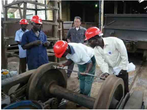
Photo 4.2.105 Measurement of Back Gauge
