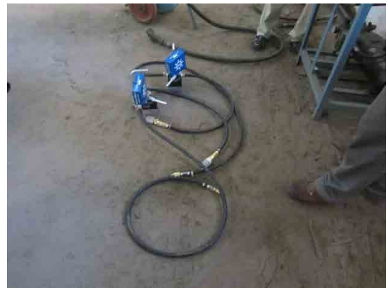
Photo 4.2.88 Assembly by Brake Test Equipment (Connecting the test equipment with the hose)
