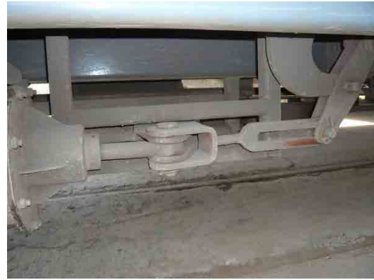
Photo 4.2.134 Brake Cylinder and Lever (with scoring traits)
