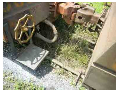
Photo 66 Defective brake hose
