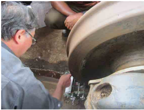
Photo 4.2.111 Measurement of Wheel Tread (Demonstration)
