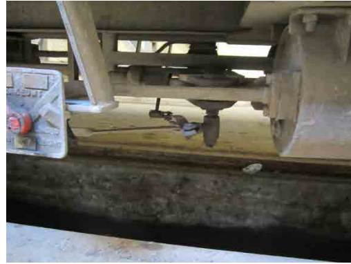
Photo 4.2.96 Non-movable Brake System which does not Move due to Sticking
