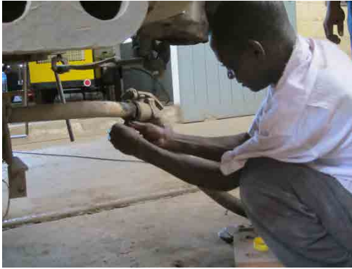
Photo 4.2.95 Repair of the Brake Pipe from Air Leakage
