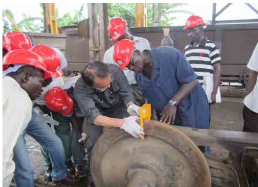
Photo 4.2.109 Measurement of Wheel Flange Measurement
