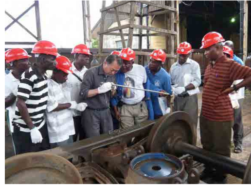
Photo 4.2.106 Measurement of Back Gauge
