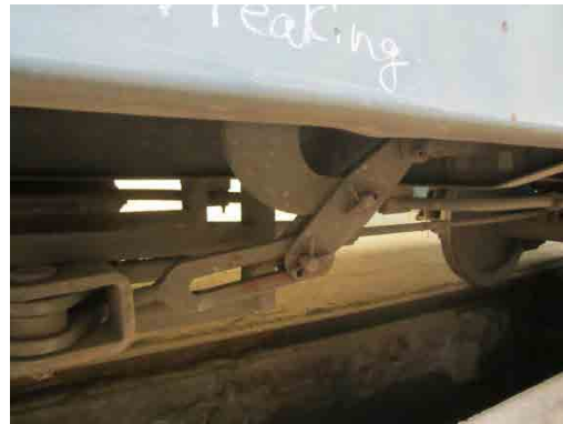
Photo 4.2.98 Check of Functionality of Brake Cylinder Lever
