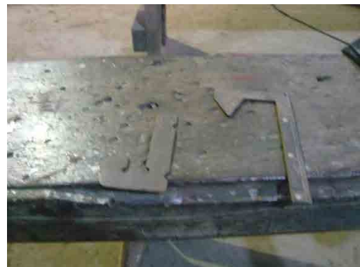
Photo 4.2.110 Old-type Flange Measurement Device Used in Ghana
