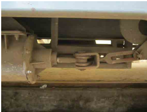
Photo 4.2.97 Check of Functionality under Brake Cylinder Released Status
