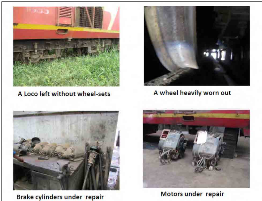
Photo 2.3.50 Defective of Locomotives
