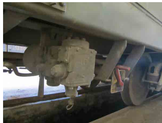
Photo 4.2.132 Brake Valve Covered with Dust
