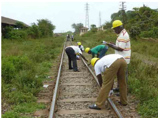
Photo 4.2.58 Each group is measuring the track irregularity
