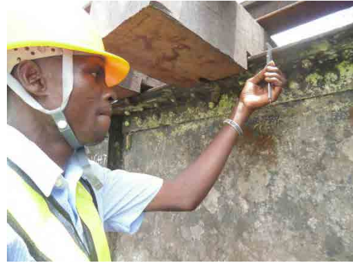
Photo 4.2.19 Thickness Measurement by Caliper (2)
