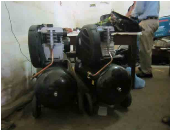
Photo 4.2.83 Brake Test Equipment Components (Compressor purchased in Ghana)
