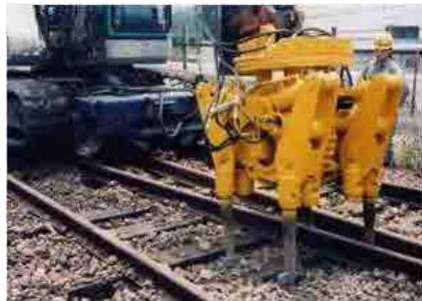
8 tools tamping equipment which is changed from the bucket attachment of road/rail Yumbo machine
