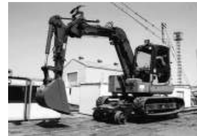
The bucket of road/rail Yumbo machine is changed to the attachment for changing sleeper. (Japanese Railway Company uses this type)
