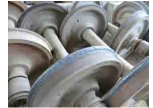
Worn tires are reused by overlay welding
