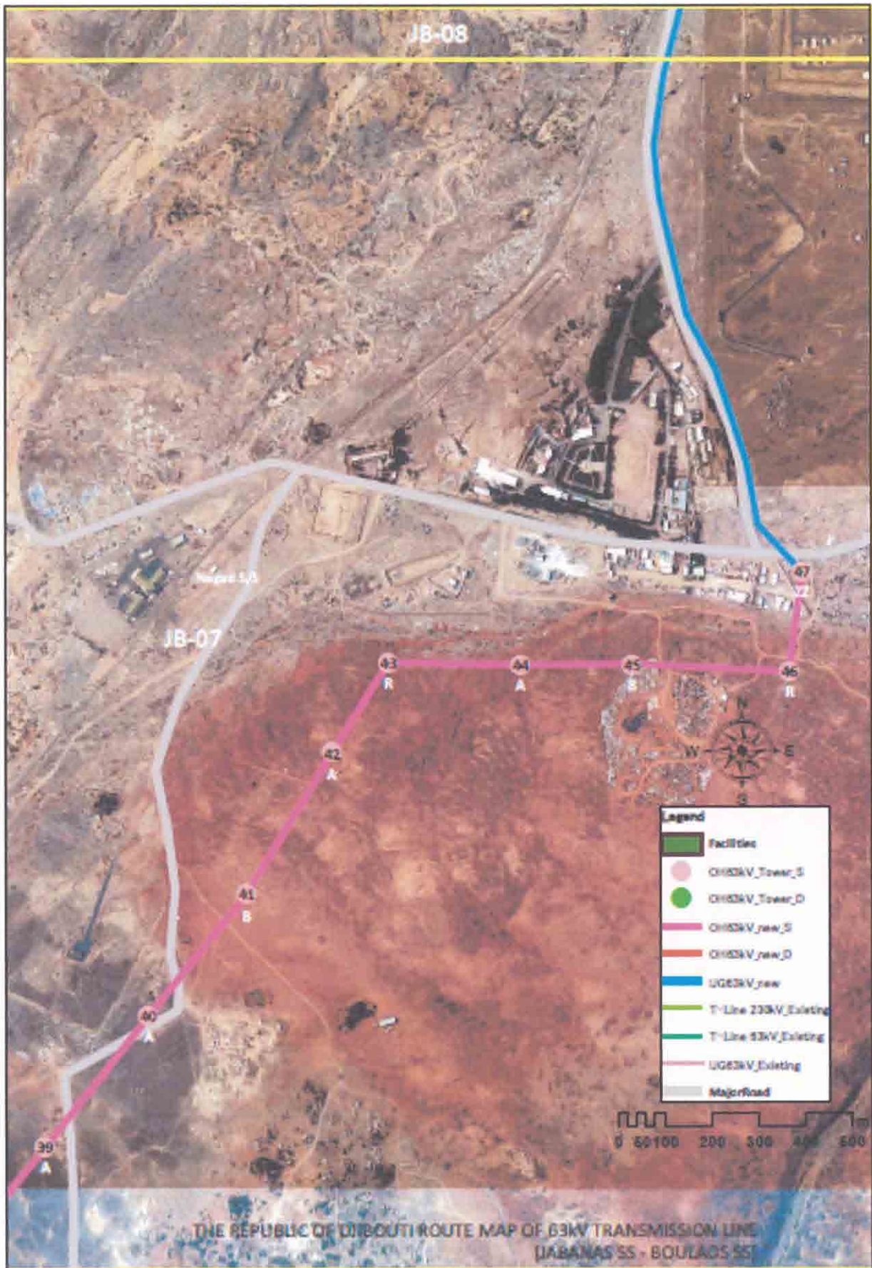
Details of Transmission Line Route (JB-07)
