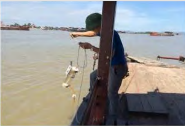
Ph-21 River near Dam Nha Mac area Surface water in the Chanh River is sampled
