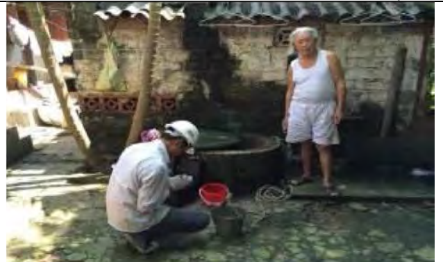
Ph-24 Tien An Area Groundwater (well water) collection and analysis
