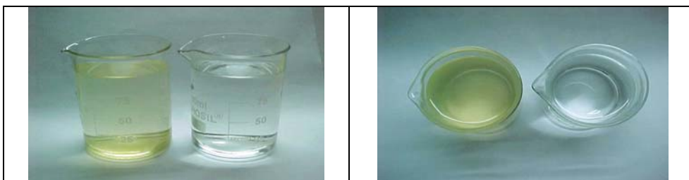
Figure 10.5 The water supplied by the WTP before (left beaker) and after the modification (right beaker) shown in side view and top view
