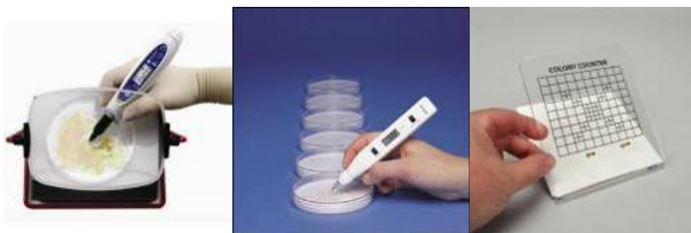
Figure 7.6 Colony counters: automatic integrating pen type and grid plate for manual use
