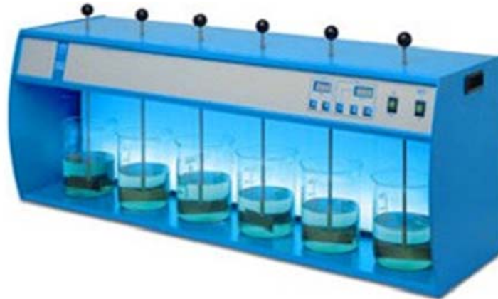
Figure 4.15 Typical jar testing apparatus
