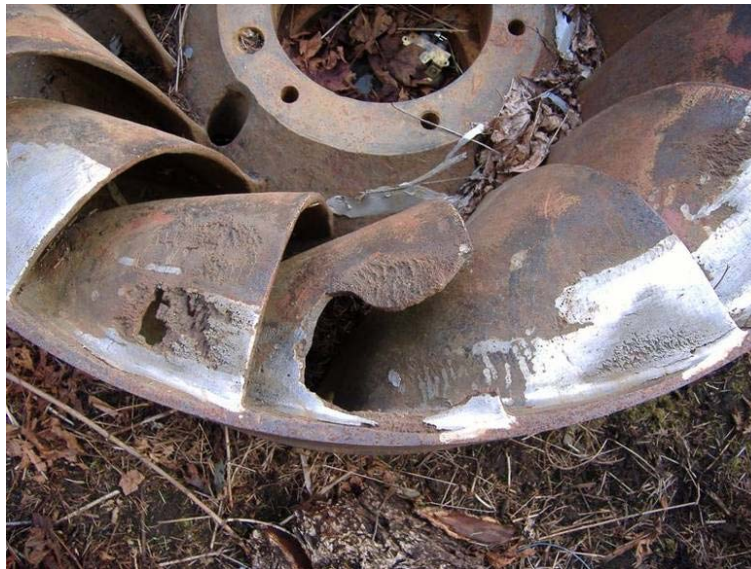
Figure 3.2 Typical cavitation damage of an impeller
