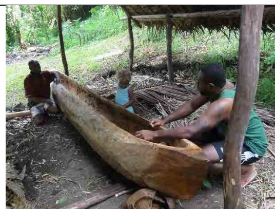
The canoe has been carved out of a log and is being prepared for construction (January 2014)
