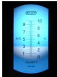
Pic14 Check salinity of the seawater at the sand filter drain pipe.
