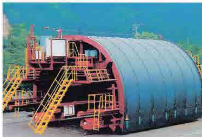
PHOTO 10.4-4 SLIDING STEEL FORM
