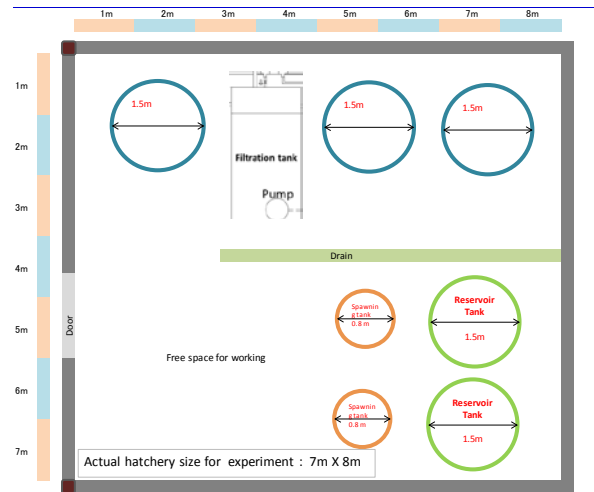
Figure 7.5 Actual tank layout
