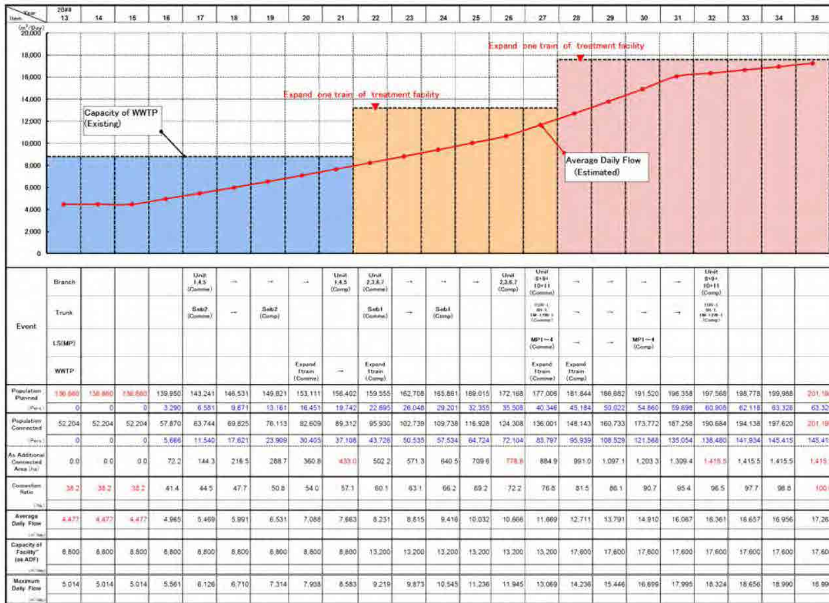
Figure 7.10 Estimated Service Population and Inflow to the WWTP and Design Capacity Improvements of Ramtha WWTP
