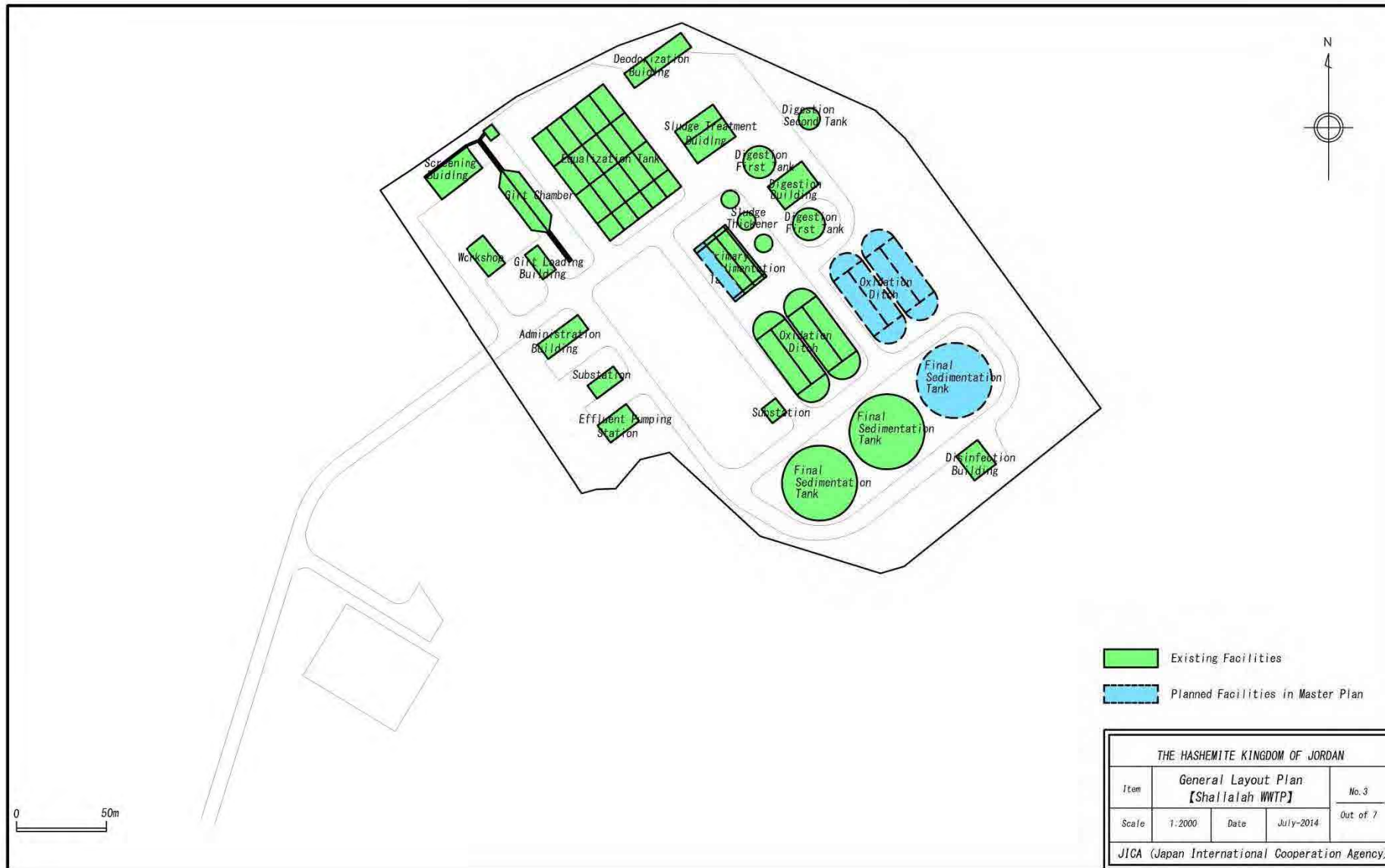
Figure 5.10 Layout of Shallalah WWTP
