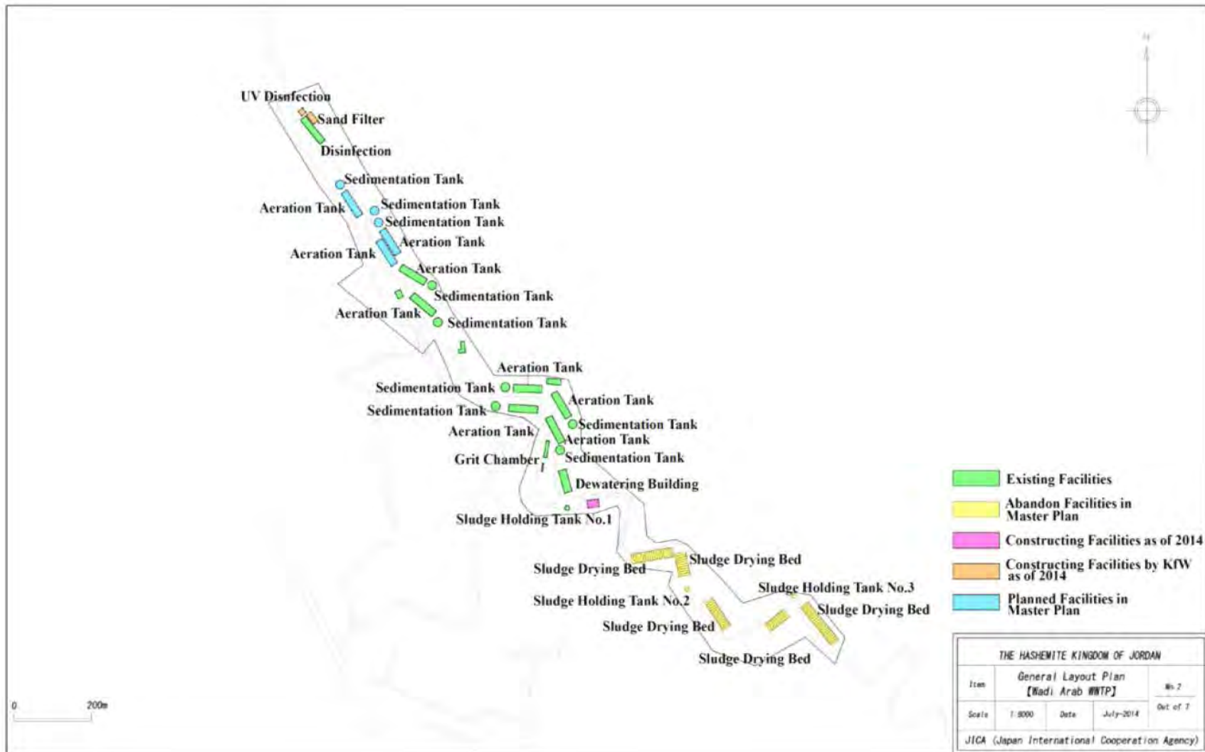
Figure 5.7 Layout of Wadi Al-Arab WWTP
