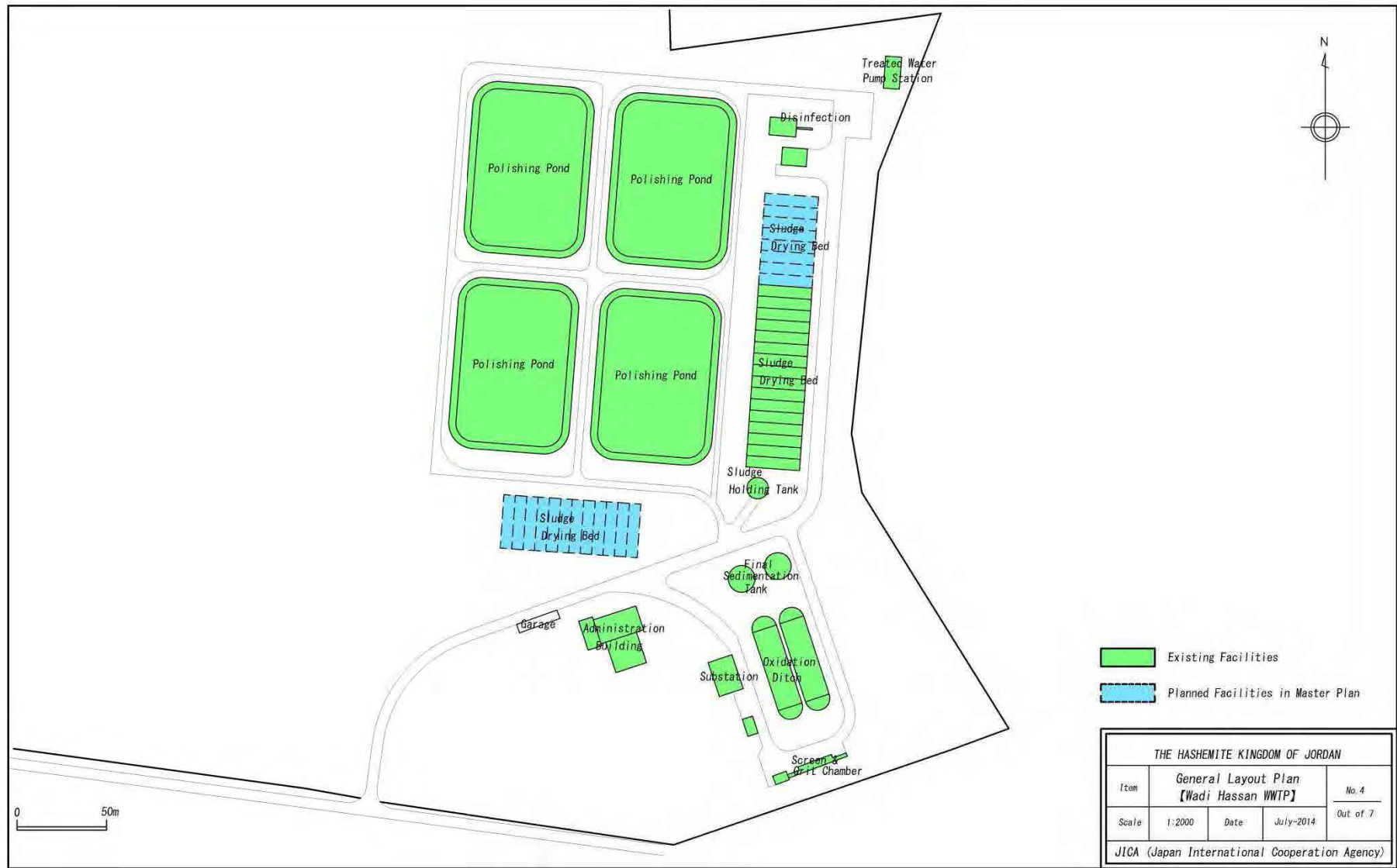
Figure 5.11 Layout of Wadi Hassan WWTW
