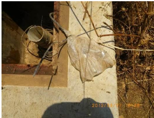
Broken Automatic Recorder for Groundwater Leveling at GN215 in 2012
