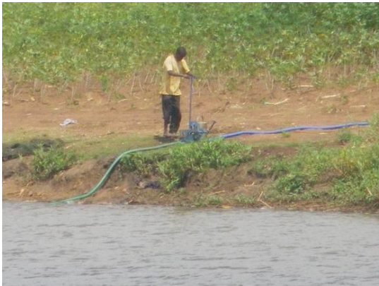
Treandle Pump at Nsandula Reservoir
