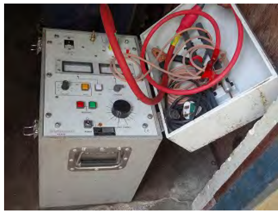
AC Withstand tester (T&R Test equipment KV30-40)
