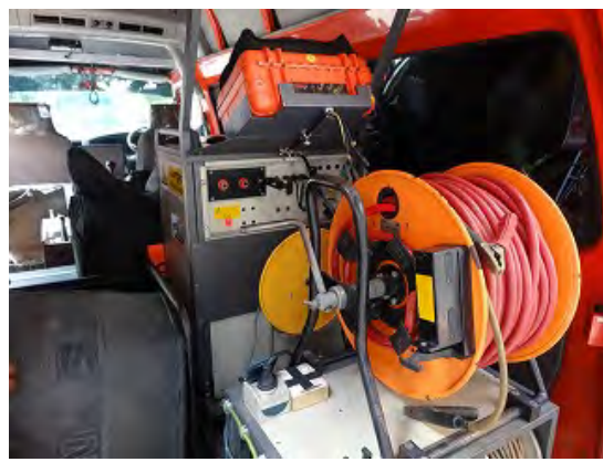
Testing and Fault Locating Unit (sebaKMT SPG32)
