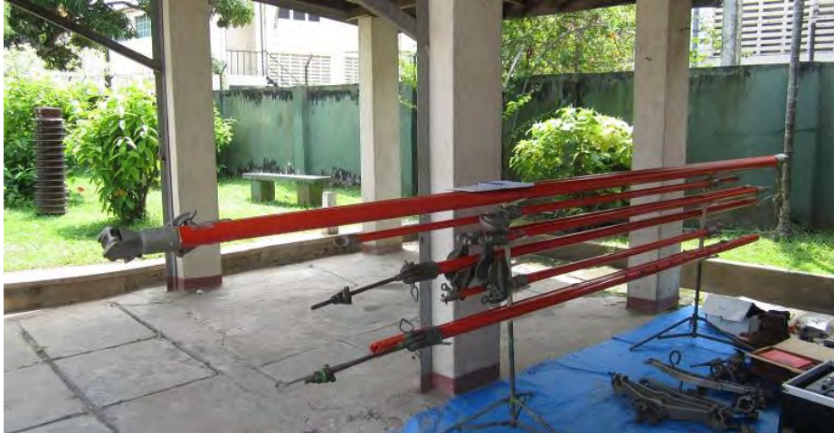
Figure 6-3 Stick Tool for hot line (Dielectric strength is 100kV/feet. According to product catalog, minimum length to keep safety is 1.09m for 132kV and 1.59m for 220kV and CEB keeps this length when they use this tool.)
